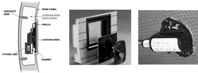
Fig. 4. Components of the Ultra electronics system of active noise cancellation "UltraQuiet"
