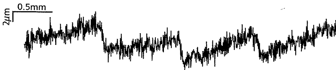
Figure 2: Profile of a milled surface.
