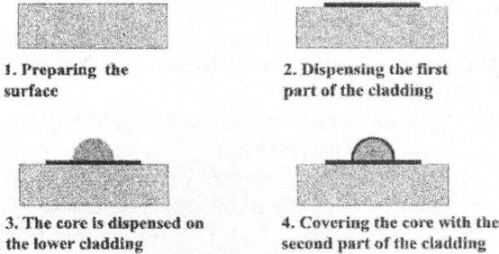
Picture 5 Creating of surface integrated light guiding structures
