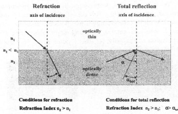
Picture 1 Refraction and total reflection
