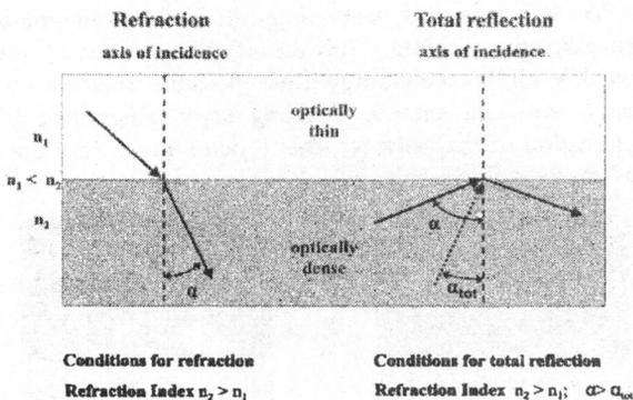
Picture 1 Refraction and total reflection
