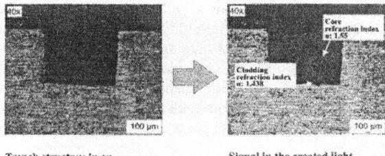
Picture 6 Surface integrated light guiding structure
