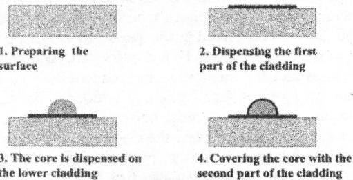
Picture 3 Creating of light guiding structures on surfaces
