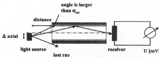
Picture 8 Influence of the misalignment of electro-optical components and light guiding structures
