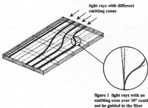
Picture 9 Simulation with a ray-tracing program
