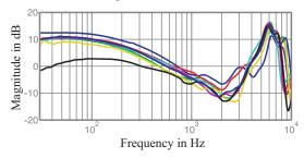
FIGURE 3. Magnitude of frequency response of the secondary paths of the test group.
