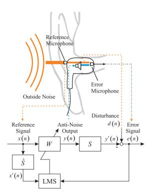
FIGURE 2. Modelling and control diagram of the adaptive feedforward control of in-ear headphones
