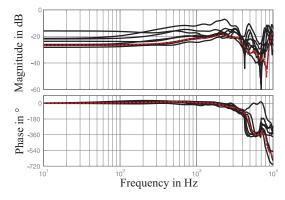
FIGURE 4. Black: Bode plot of the adapted filters of the FxLMS-algorithm for the test group; dotted red: static filter
