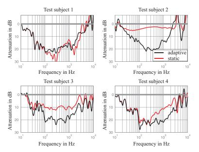
**FIGURE 5.** Comparison of active attenuation of the adaptive and static feedforward for different test subjects. The adaptive attenuation is plotted in black and the static attenuation in red.
