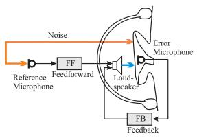
FIGURE 1. Combined feedback and feedforward control of supra-aural headphones.
