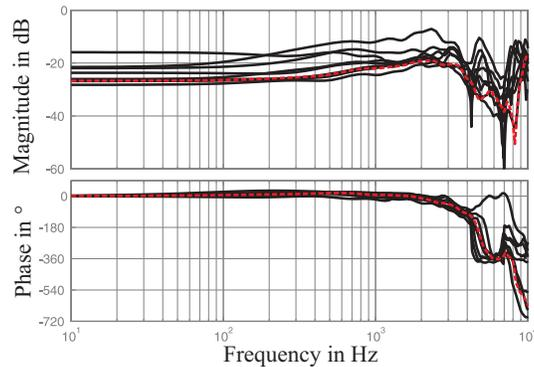
**FIGURE 4.** Black: Bode plot of the adapted filters of the FxLMS-algorithm for the test group; dotted red: static filter
