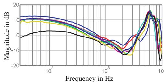
**FIGURE 3.** Magnitude of frequency response of the secondary paths of the test group.
