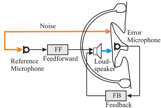
**FIGURE 1.** Combined feedback and feedforward control of supra-aural headphones.
